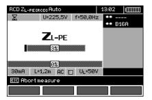
Progress of measurement process is shown by progress bars:
