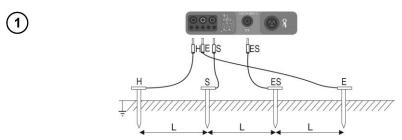
Four probes driven into the ground along one line and in equal distances must be connected as shown in the picture above.
