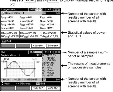
Press F3 and F4 Screen to display the results of measurements in successive samples.
