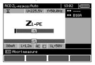
Progress of measurement process is shown by progress bars: bottom - the whole cycle, upper – Z<sub>L-PE</sub> RCD measurement and RCD parame-
