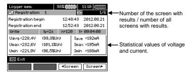
Press F3 | ◆Screen | and F4 | Screen | to display individual results for a given rec-
