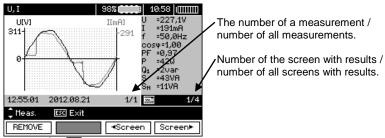
Use ▲, ▼ to display the results of subsequent measurements.
