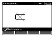
Batteries /rechargeable batteries are fully discharged, the measurement is stopped.
