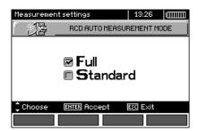
In the standard mode, measurements are performed for a selected current waveform, in the full mode for all current waveforms of a given type of RCD (AC, A, B, B+, F).
