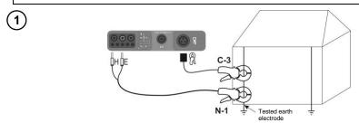
Transmitting clamps and measuring clamps should be attached to the tested earth electrode at a distance of at least 30 cm from each other.
