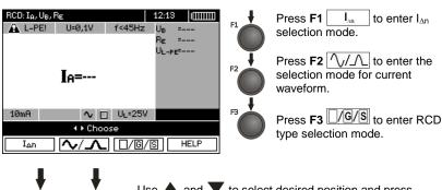
Use **A** and **V** to select desired position and press **ENTER** to confirm.
