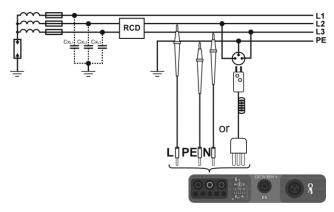
a) Parasitic capacitance is used during the measurement.
