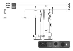
The way of making short circuit loop measurements is described in point 3.4.1. Operating voltage range:  $95 \text{ V} \dots 440 \text{ V}$ .
