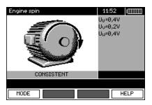
The arrow rotates counter-clockwise: when L1, L2, L3 motor terminals are connected to L1, L2, L3 phases (respectively), the motor will rotate in the opposite direction to the rotations during the test.
