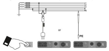
After connecting the meter according to the drawing, touch the contact electrode with a finger and wait for about 1 second. When voltage is found on PE the meter displays **PE!** symbol (error in the installation; PE connected to the phase conductor) and generates a continuous beep. This option is available for all measuring functions that apply to residual current devices (RCD) and fault loop.
