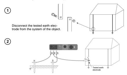
The current electrode (driven into earth) should be connected to **H** socket of the meter.
