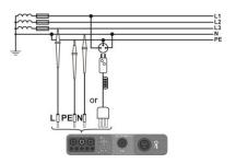
Measurement in L-PE circuit
