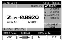
Read out the result:  $Z_{L\text{-PE}} \text{ - the main result } I_a \text{ - current ensuring automatic triggering of a selected protective device in a required time } I_k \text{ - prospective short-circuit current } R, X_L, U_{L\text{-PE}}, f \text{ - additional results.}$
