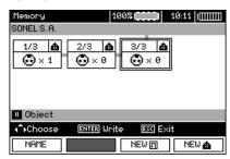
To add a new sub-object, set the cursor on the chosen object and press F3
