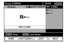
AUTOZERO message appears that confirms completion of test leads calibration.
