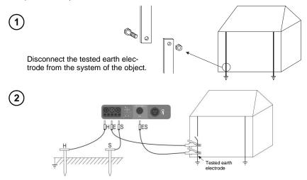
The current electrode (driven into earth) should be connected to **H** socket of the meter.
